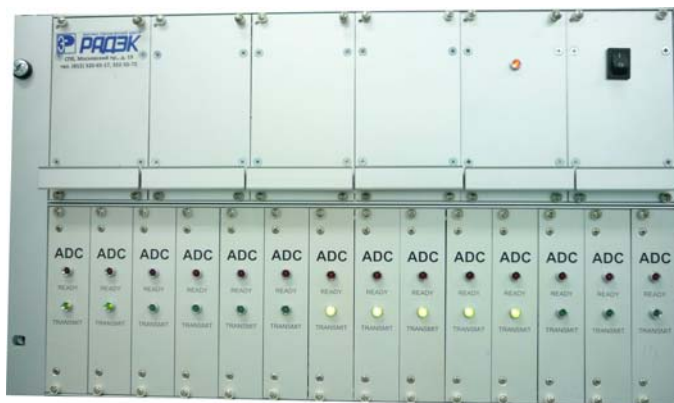
Fig.6. View of 14 analyzers MD-198 from the front side in the control cabinet.
